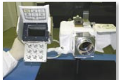
The protective housing for the ThermaCAM S65 as developed by NASA
